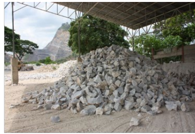
Rocks that have been shredded and prepared for use as raw materials for calcium carbonate production.
