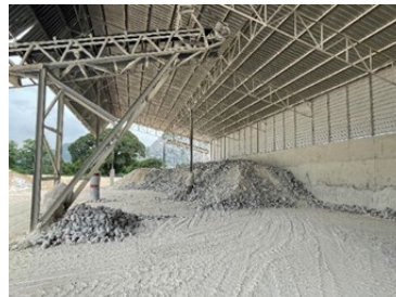
Rocks that have been shredded and prepared for use as raw materials for calcium carbonate production.
